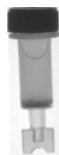
Figure 5. Zeba™ desalt spin column used to rapidly exchange or desalt samples. Zeba™ columns have a maximum loading capacity of 130 ul.
